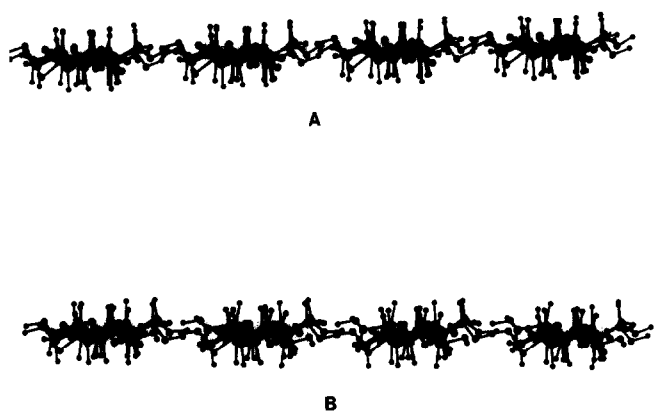
Figure 2 A glucan mini-sheet along the (010) plane of cellulose I \beta before (A) and after (B) energy minimization at \epsilon = 4 . The small degree of molecular movement indicates the model is stable at this dielectric constant
